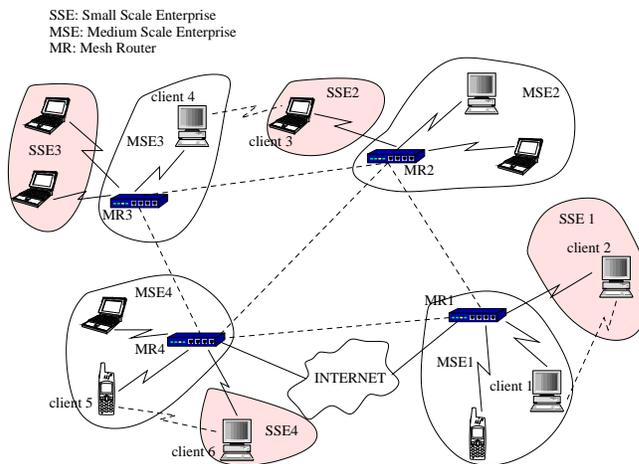
Figure 2: Operator-less Collaborative Network
