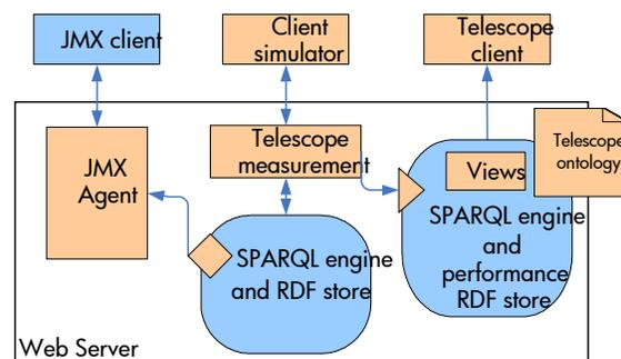
Figure 1 - Architecture for our management and monitoring framework.
